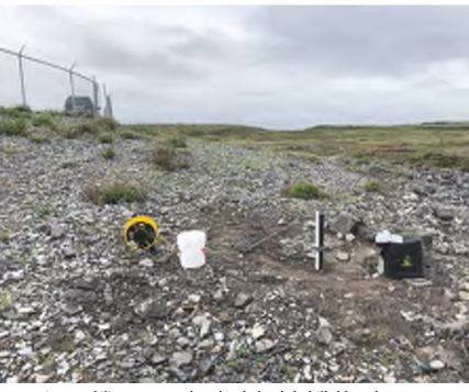
A permeability test was conducted in the borehole drilled from the western sideslope. A levelogger was programmed and lowered into the one-inch slotted standpipe. The standpipe was filled with water, and the water level versus time was logged. A water level tape was used as a backup measurement. The data has been compiled to provide a comprehensive picture of the ground conditions within the lagoon system to development schematic designs for remediation work.
